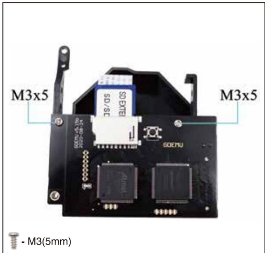
2. Use the included M3(5mm) screws to fix the GDEMU on the bracket, and Plug the SD Card Ribbon cable into the GDEMU.
