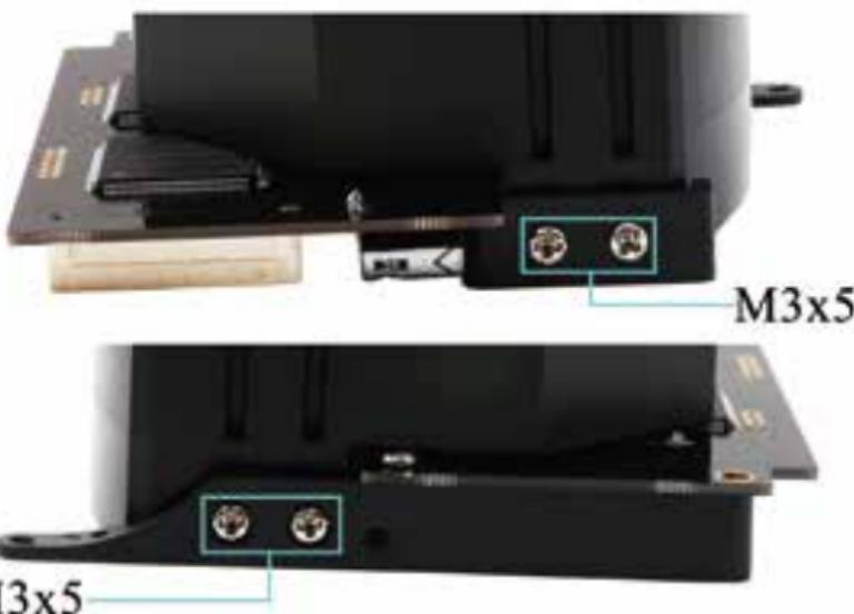
3. Put the top box,bracket set and the next disc button together, and fix them with screws.
