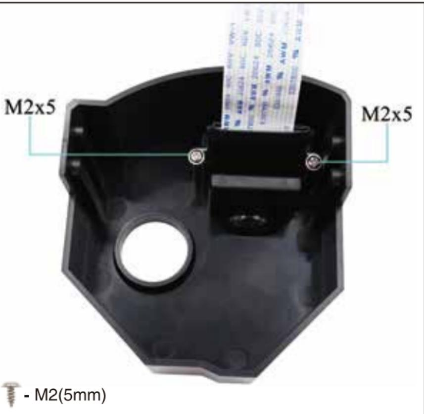
1. Use the included M2(5mm) screws to secure the SD Card Ribbon cable to the top box.
